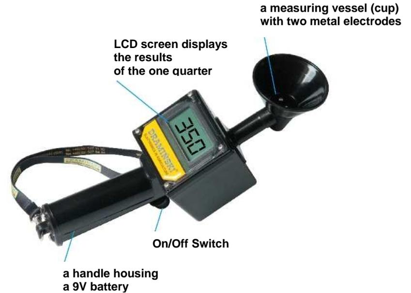
The device housing is drop-proof what makes its use more safe and cleaning easier.
